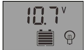
④ load disconnect voltage
